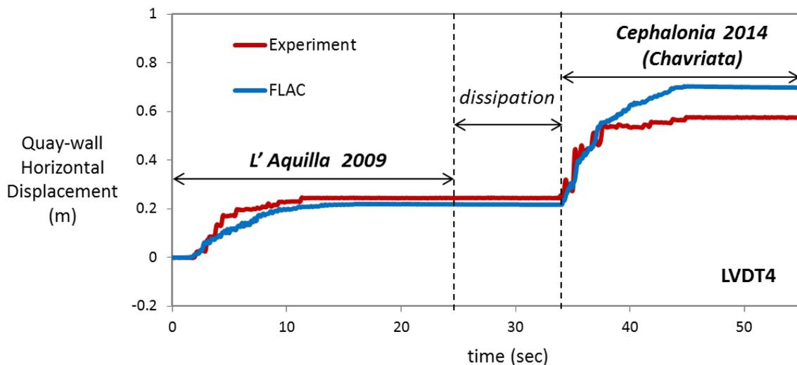
**Figure 5.** Predicted quay-wall outward horizontal displacement at top (location LVDT4 in Figure 1).
