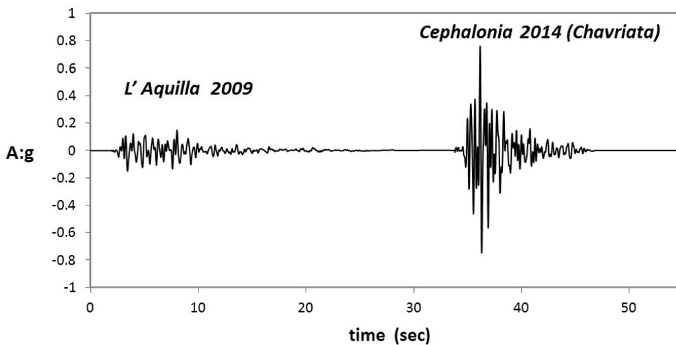
**Figure 2.** Acceleration time history of input motions applied at the base of the model
