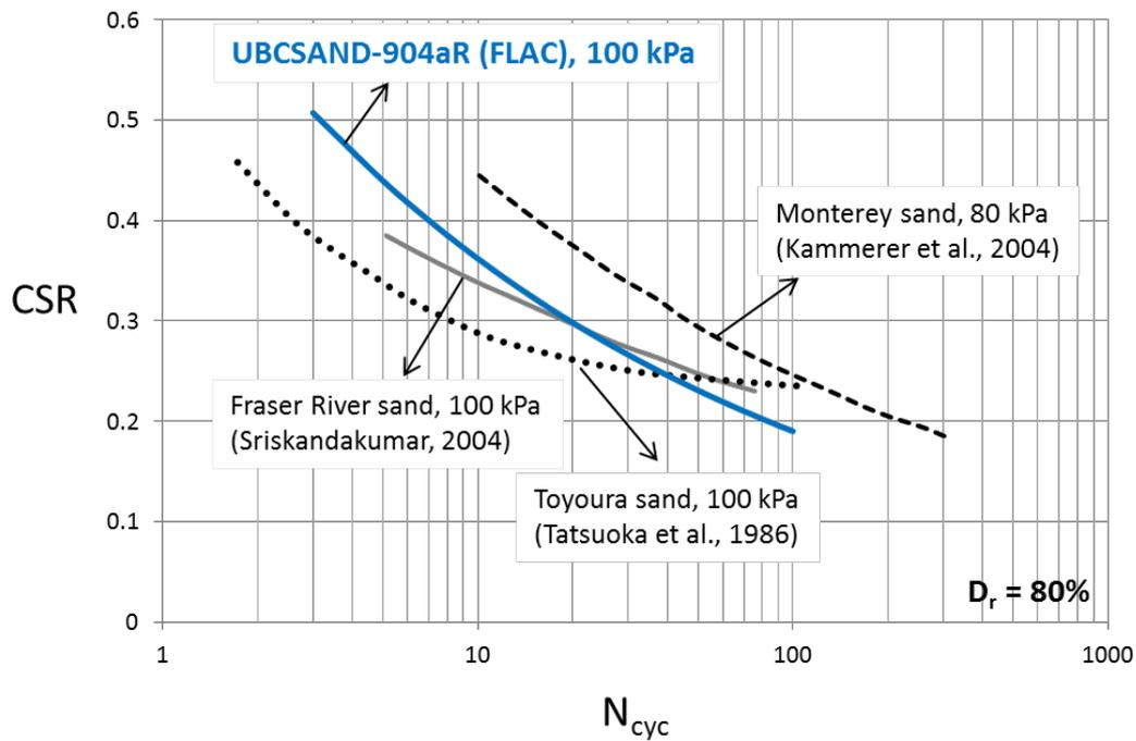
**Figure 4.** Comparison between predicted and experimental liquefaction resistance curves in undrained cyclic simple shear testing for  $D_r = 80\%$ .
