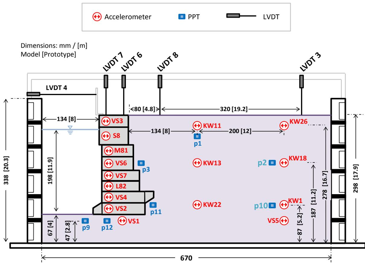
**Figure 1.** Centrifuge model setup and instrument locations
